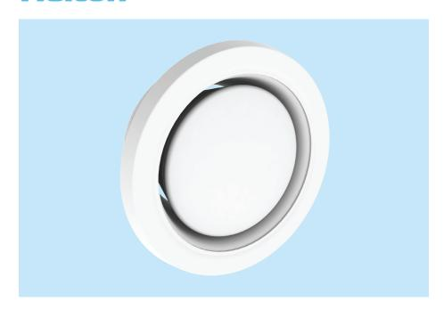
The Halton FDV, which has replaced the Halton FRH, is a circular fire valve, which combines an exhaust valve and fire damper for the ducts. FDV is designed to prevent fire and smoke from spreading in ventilation ducts.
