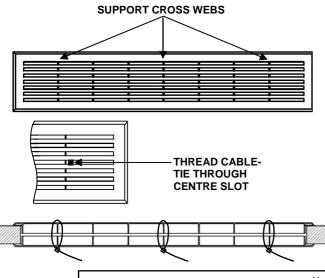
6. With a flat-head screw driver, push the head of the cable-tie through the gap, whilst pulling on the tail end to tighten grilles together, or use long nose pliers to pull and tighten the cable through the centre slot.
