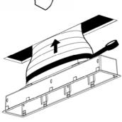
4. Pass the boot up through the hole in the ceiling and insert the plastic clips into the clip holes. Ensure the clips are pushed through as far as possible and that the boot width is not distorted.
