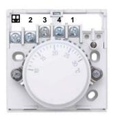
NOTE: Terminal 4 is the 'make on temperature rise' contact; this can be used to power a 'cooling' ventilation fan. Please note you can't wire both heating and cooling to the same thermostat.
